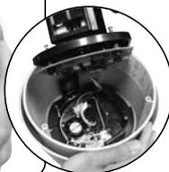
Carefully lift up the camera base from the casing.
