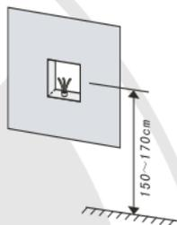
2. Fix the mounting plate to the wall, using the screws supplied (see Fixing Holes Guide). Drill a hole in the centre of the mounting plate large enough to feed the cables through.
