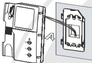
5. Insert the securing screw into the hole on the top of the mounting plate to secure the handset.
