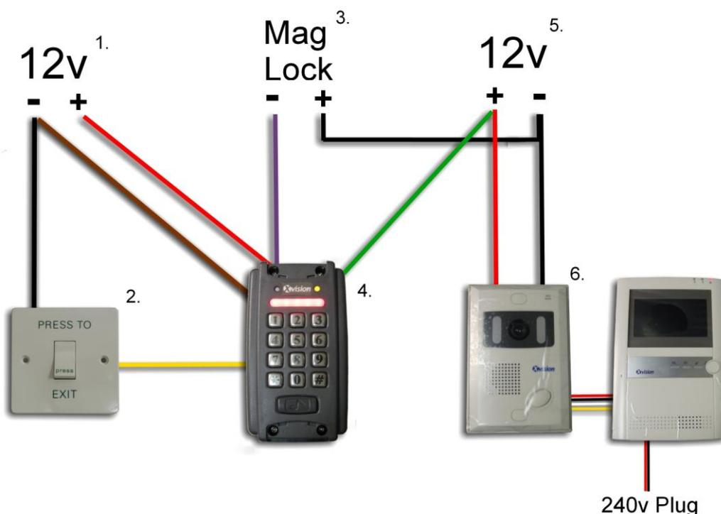
**Step 2: Connect the XD100 (4) using the 6 pin cable**
