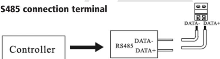
Use the RS485 port to connect the camera to a keyboard controller and control it. The camera is compatible with eight different protocols.
