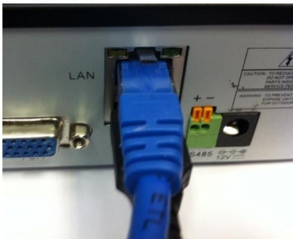
**Step 2:** Plug the Ethernet cable (supplied) into the LAN port on the back of your IQR960 DVR.
