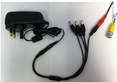
**Step 2:** If you are using a power splitter cable to power multiple cameras on one power supply connect the red DC power socket on the other end of the 18m video cables (labelled TO DVR SIDE ONLY) to one of the 4 plugs on the power splitter. Then connect the single DC power socket end of the 4 way power splitter to the DC power supply (supplied with the camera) as illustrated to the left.
