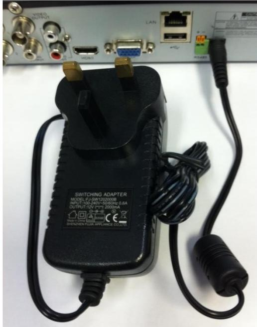
**Step 3:** Plug the DVR power supply into a suitable mains socket
