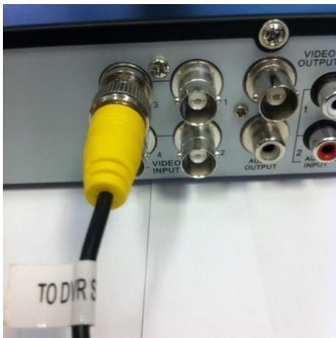
**Step 3:** Connect the yellow video output BNC plug (labelled TO DVR SIDE ONLY) to the VIDEO INPUT socket on the back of the IQR960 DVR.
