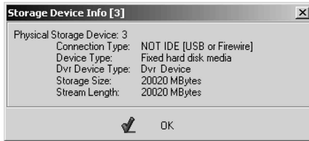
Fig.4. DVR Storage Device Information Window
