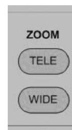
Zooming of the camera can be controlled by the Zoom function. Use the TELE (Zoom in) and WIDE (Zoom out) keys on the keyboard controller.
